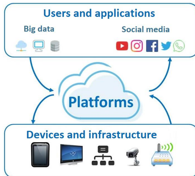
Figure 4 – Simplified IoT layered architecture.
