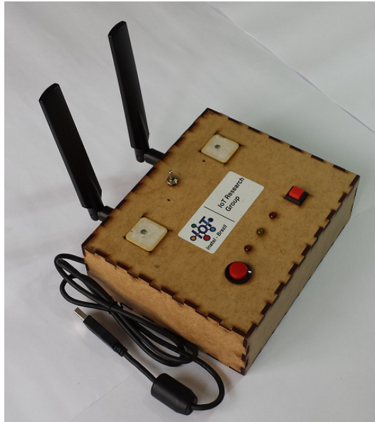
FIGURE 3.11: Assembled Equipment with LoRa and Sigfox Terminal Devices.
