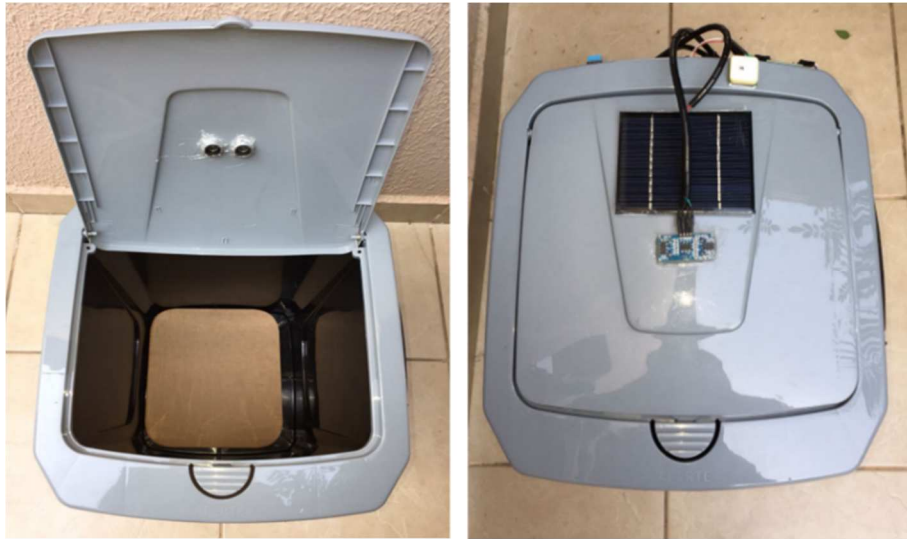
Figure 14.a: Smart bin's internal image. Figure 15.b: Smart bin's internal top image.
