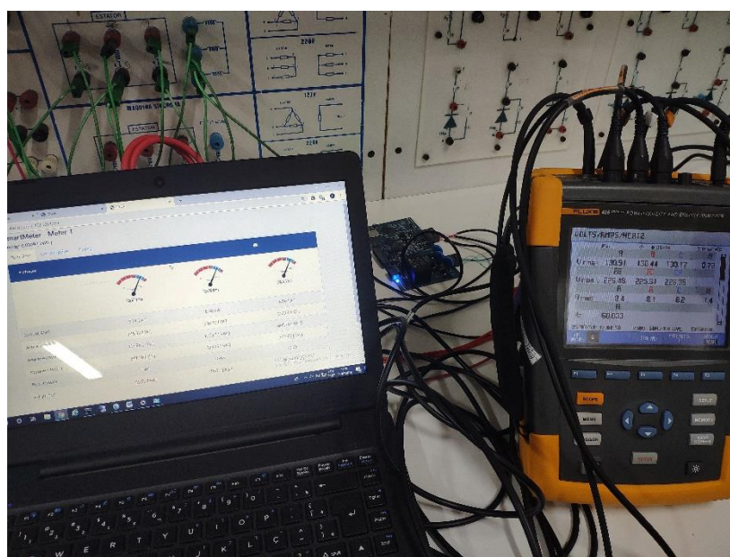
Figure 18 - Comparison of measurements between the smart energy meter and a commercial meter.
