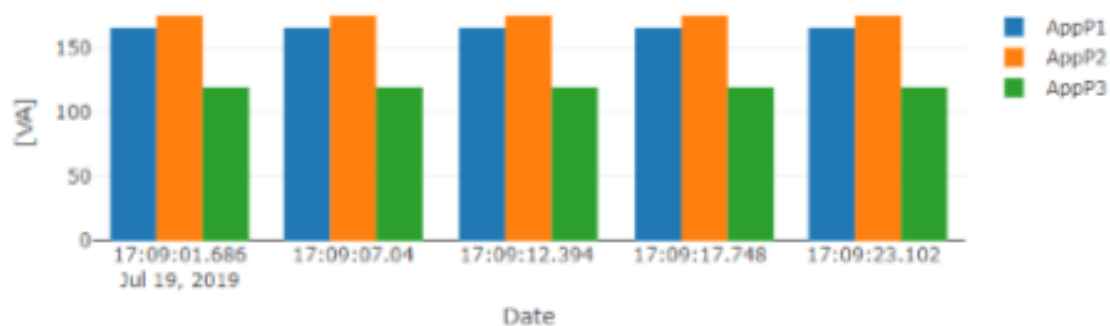
Figure 15 - Status of Apparent Power variable measured by the smart energy meter in real time via Web - In.IoT
