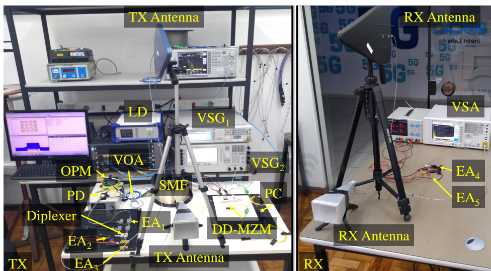
Fig. 6. Photography of the experimental setup.
