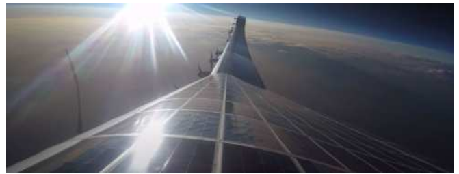
FIGURE 5. “Sunlider” HIBS Platform flying at the stratosphere during an LTE video call communication test between United States and Japan. [Courtesy of HAPSMobile/Loon].
